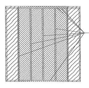
Use a minimum 1 1/2 inch long drywoll screws, nails or staples at 6 inches on center along the panel edge and 12 inches on center in the field to the framing members. It is particularly important to pay attention to these details at the top and bottom of the applied panel.
