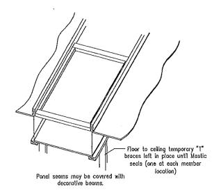
STEP 3: Secure the replacement panel to the framing using 3/8" bead of glue applied to all perimeter and Field framing members.
