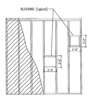
Damaged Wall board "patch" material sholl be an equivalent thickness of gypsum
