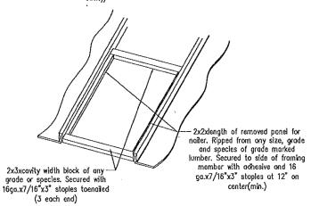
STEP 2: Add a 2x3 (min.) block at each end of the removed panel to provide a surface for attachment of the new panel.
