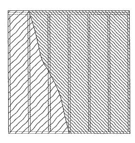
Any interior wall surface may be overlaid with an additional gypsum wall panel in lieu of removing the existing panels. The overlay panel must be securely fastened. The fastener length is to be increased by a minimum of the thickness of the gypsum panel being overlaid.
